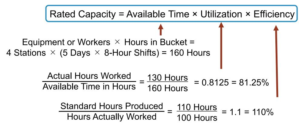
Rated Capacity = 160 Hours  $\times$  0.8125  $\times$  1.1 = 143 Hours
